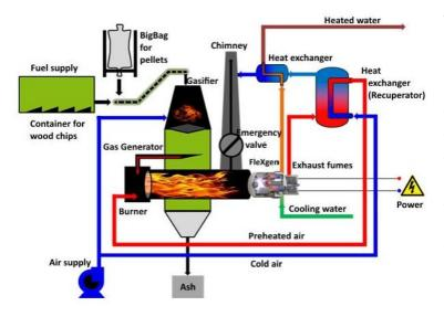
The chute is superimposed of the Barrier gas air principle. Also, a slider, which is opened only for the charging process, prevents in a standard case the exit of producer gas upwards into the chute. With a level sensor inside the fixed bed reactor the loading operation will be initialized and terminated.
