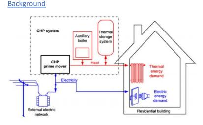
CHP (Combined Heat and Power) are systems that produce electrical and thermal loads at the same time. Until recently the production of electricity was made in power plants where huge amounts of heat energy were lost in the environment. The principal idea of CHP is to take advantage of the thermal energy from the production of electricity. Thus, CHP are high efficiency systems.
